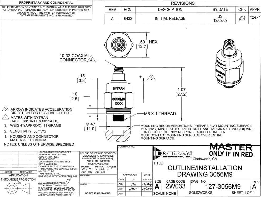
Model Number DOC NO PERFORMANCE SPECIFICATIONS 3056M9 PS3056M9 IEPE ACCELEROMETER REV C. ECN 7932, 10/12/11
