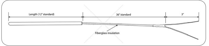
Thermocouple calibration type N is available in all sizes.
